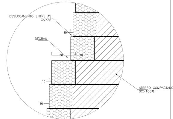
DETALHE 1: SAÍDA DA DRENAGEM INTERNA SEM ESCALA
